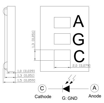
Note: 1. All dimensions are in millimeters(inches) 2. Tolerances unless dimensions ± 0.25mm (.01")
