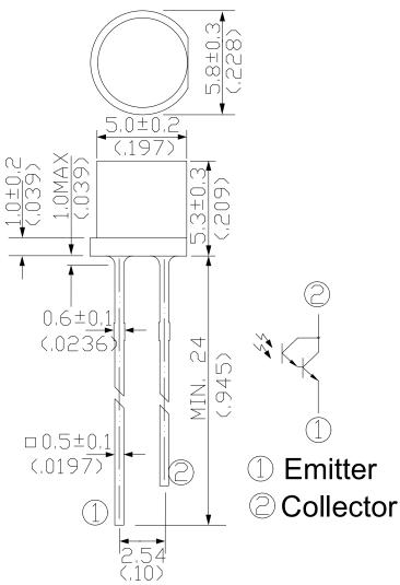
Note: 1. All dimensions are in millimeters(inches) 2. Tolerances unless dimensions ± 0.25mm(.01")
